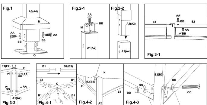
Fig 1: Let Stake Cover (N) go through pole (A3, A4). Then attach Lower Post (A3, A4) to Piece for stakes (O) with screws.
